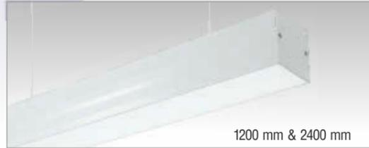
LED luminaire having 95 mm wide aluminum extruded profile finished in white powder coated. Snap fit high translucent frosted PMMA diffuser and high reflective aluminum reflector gives glare free light distribution with maximum efficiency. Another advantage of this system is the complete flexibility of continuous mounting which makes it adaptable to any architectural requirement and has a feature of overlapping lamp placement which results "shadow free" illumination.
