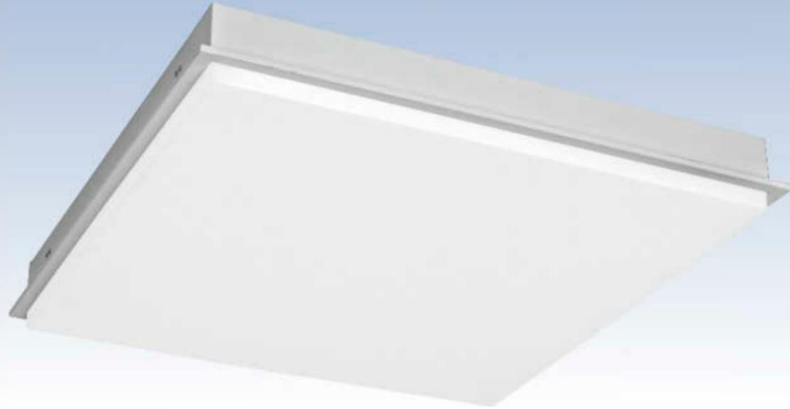
With a drop down acrylic diffuser the Arion III is designed to be a aesthetical icon to convert your ceiling space into a piece of art. With the aesthetic brilliance without compromising on the photometric performance the Arion III is an ideal ceiling solution of the grid type ceilings. The Arion III is constructed of CRCA Sheet metal housing and a premium quality drop down PMMA diffuser making it an ideal choice for office lighting.
