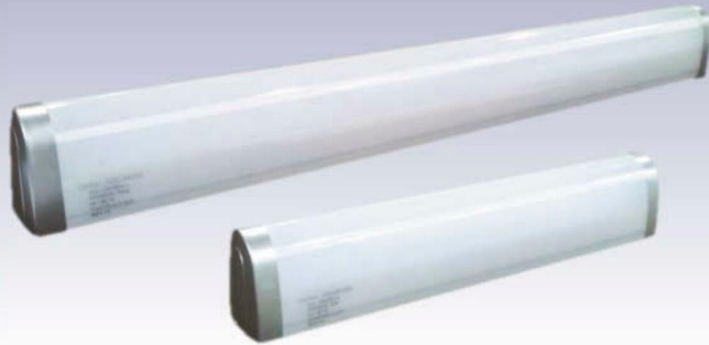
LED luminaire comprises of aluminium extruded channel finished in anodised with Silver painted plastic end cap. The luminaire is pre-wired with high efficiency electronic driver. High translucent frosted PMMA diffuser is used to get glare free, smooth light distribution. Luminaire is recommended for corridor lighting, home lighting, task lighting etc.
