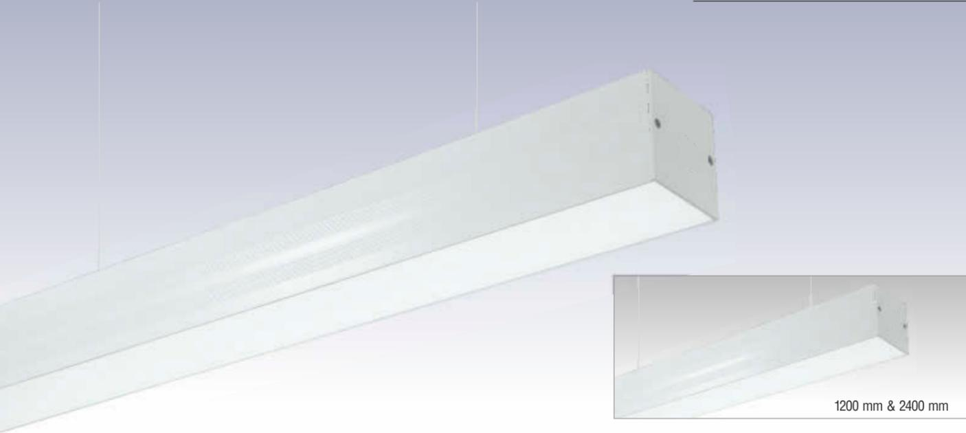
LED luminaire having 95 mm wide aluminum extruded profile finished in white powder coated. Snap fit high translucent frosted PMMA diffuser and high reflective aluminum reflector gives glare free light distribution with maximum efficiency. Another advantage of this system is the complete flexibility of continuous mounting which makes it adaptable to any architectural requirement and has a feature of overlapping lamp placement which results "shadow free" illumination.
