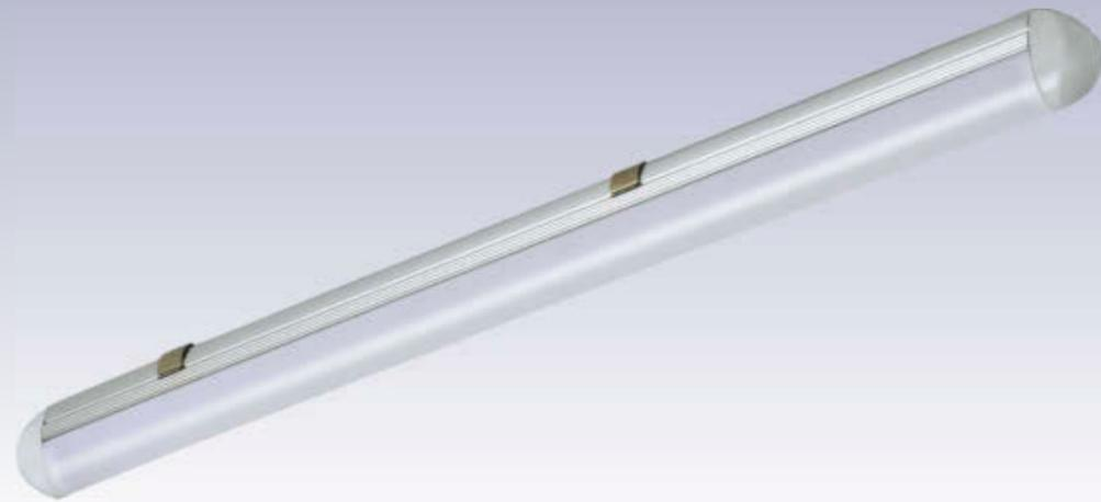
This LED luminaire comprises of extruded channel in thermally conductive material with decorative plastic end cap. The luminaire is pre-wired with high efficiency electronic driver. High translucent frosted diffuser is used to get glare free, smooth light distribution. The luminaire is recommended for corridor lighting, home lighting, task lighting.
