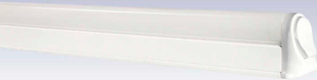
This LED luminaire comprises of co-extruded housing in Engineering Plastic with Opal serrated top diffuser used to get glare free, smooth light distribution. Injection moulded 2 piece white color plastic end cap. The luminaire is pre-wired with high efficiency electronic driver. The luminaire is recommended for corridor lighting, home, office lighting etc.
